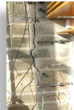
**Intermediate failure mechanism Ribalt. Composto Mec. II**
